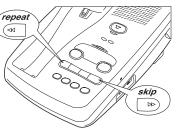
3) To set the second number, press *skip* or *repeat* to scroll from *D* to *9*. When the desired number appears in the display, press *pin*. This selects the second number and the entered PIN is announced.
